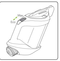
The product has 2 power settings: Max mode (higher suction power and shorter runtime) and Eco mode (lower suction power and longer runtime). Change modes by sliding the switch located in front of the On/Off button. The product will turn on in the mode it was last used.
