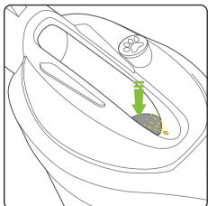
A light above the window on the top of the lid allows visibility into the bag to indicate when the bag is full or if there is a blockage.
