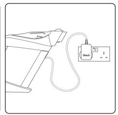
Plug the charger in and connect it to the charging port on the side of the battery.
