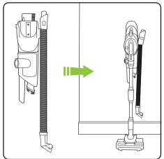
Install your wall mount at least 1072mm from the floor. Universal fixings have been included - please use the correct fixings for the wall type you're mounting this item to. Please use a stud finder to ensure no water pipes or electrical cables are hit. The tools can be stored like this on the wall mount. Your wall mount will look like the picture on the right when fully assembled with the product.
