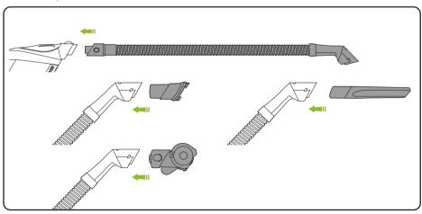
The flexible power hose attaches in the same way as the other accessories and can be used as it is or with the the addition of other tools. Powered units can fit directly to the flexible power hose.
