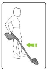
Pulling the vacuum back towards you activates the AirLOC and picks up finer particles.
