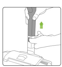
You can also remove the handle while the steering module is still attached to the main unit to use the handle with the duster.
