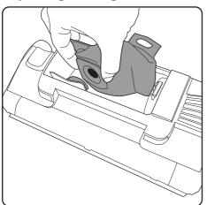
Put the new bag in the bag-chamber, fitting the collar over the inlet.
