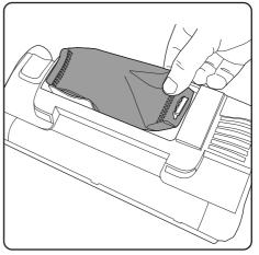
To expand the bag, pull the hoop at the end of the bag over the hook at the edge of the chamber.
