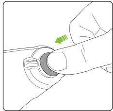
You will then need to reset the eject system by pushing the button back into place.
