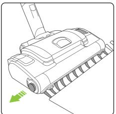
In the case of a jam, the brush-bar will automatically eject itself to allow you to remove any obstructions and prevent damages. Once the brush-bar ejects, turn the unit off.
