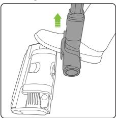
To remove the handle, hold the main unit down with your foot and pull upwards on the handle.
