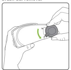
Remove the battery before maintaining any part of your product. Rotate the latch from the 'locked' position to the 'unlocked' position.
