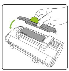
Place the lid back onto the chamber and press down. It will click into place once it is secure.
