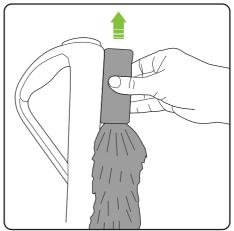
To remove the duster simply slide it upwards and off the handle.
