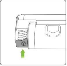
Press the power button to turn it on. You can also do this with your hand when it is in hand-held mode - be careful of the rotating brush-bar.
