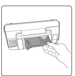
Turn the product onto its back, unhook the end of the bag and disconnect the collar from the inlet. You can then remove the bag.
